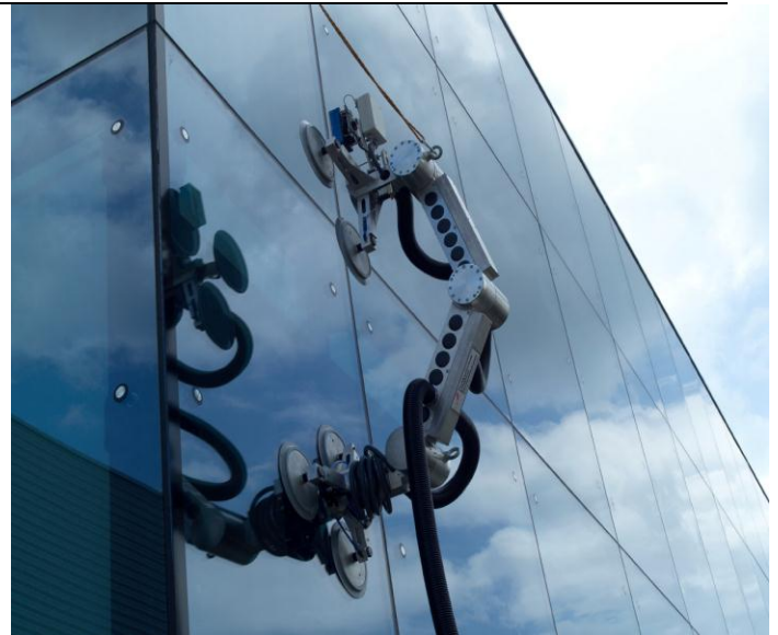
Fig. 3. Façade climbing robots for inspection and maintenance
