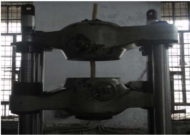
Fig. 6. Tensile Strength Test of Bamboo Stick.
