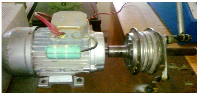
Fig 2: Motor with mechanical load.
