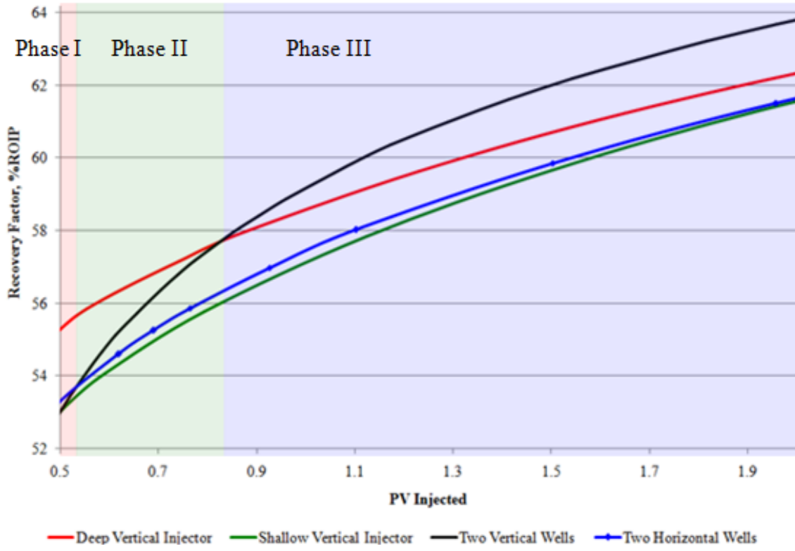
Fig. 30: Recovery Factor for Different Well Arrangement over Pore Volume Injected
