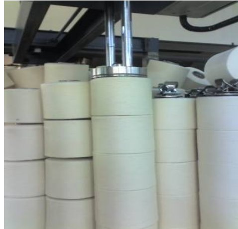
Fig-3: Dyeing carrier loaded with soft winding packages on plastic type holder where TOP CIRCLE of lower package inset into the BOTTOM CIRCLE of upper package & thus support the weight of upper package and so the lower packages gain no extra pressure from the weight of upper packages.
