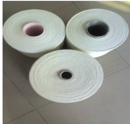
Fig: 2: (b) soft winding packages from grey package on spring and plastic tube.
