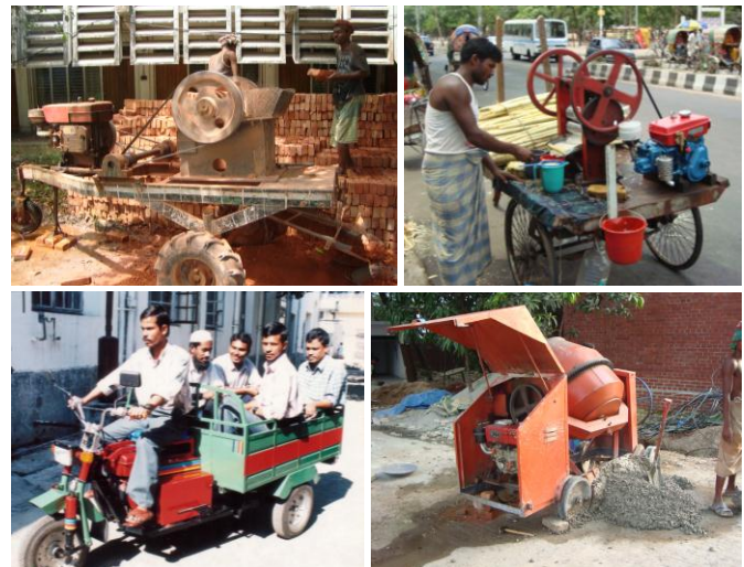
Fig. 1. Various non-conventional use of small single cylinder diesel engines in Bangladesh.
