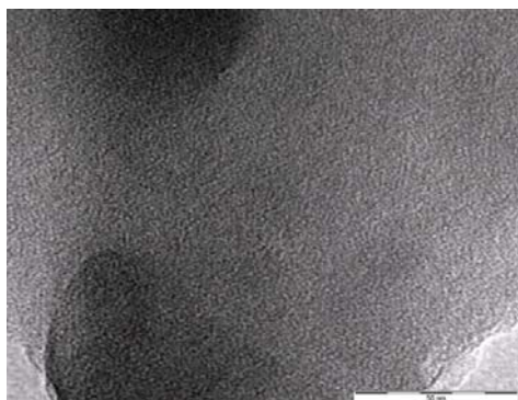
Fig. 8. TEM micrograph of CMS membrane
