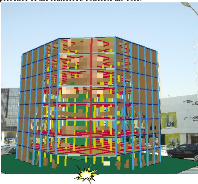
Fig. 8. Damage state of building at 3.1s
