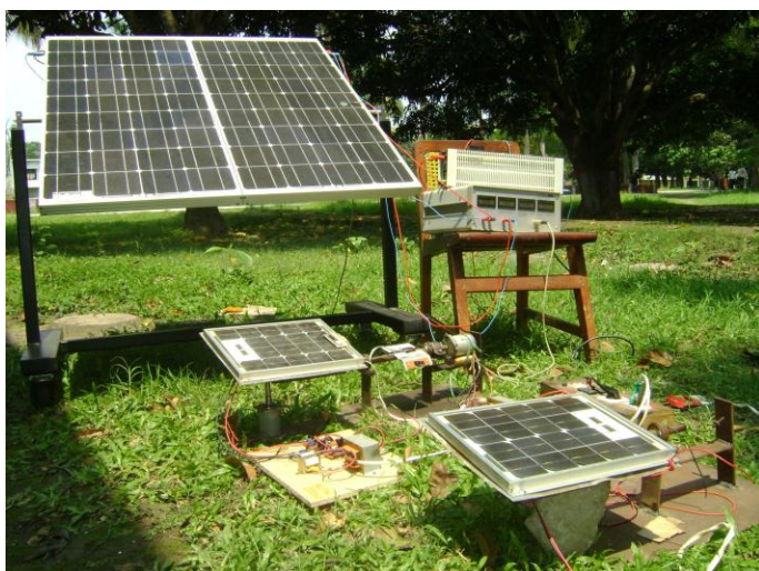
Fig. 6. Photographic of Experimental set-up of the entire system
